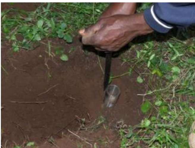
Figure 7. Taking a soil sample using a volumetric corer (Photo by J. Alm).
