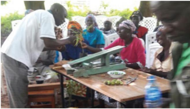
Demonstration of Melia seed cracking by use of improvised nut cracker
