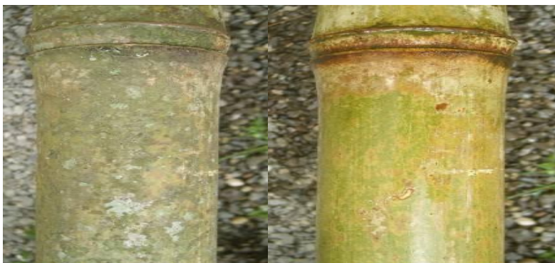
Plate 17 Left, bamboo that has not been scoured and right bamboo that has been scoured
