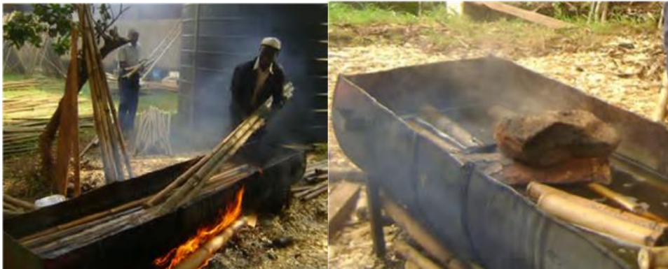
Plate 20: Treatment of bamboo culms
