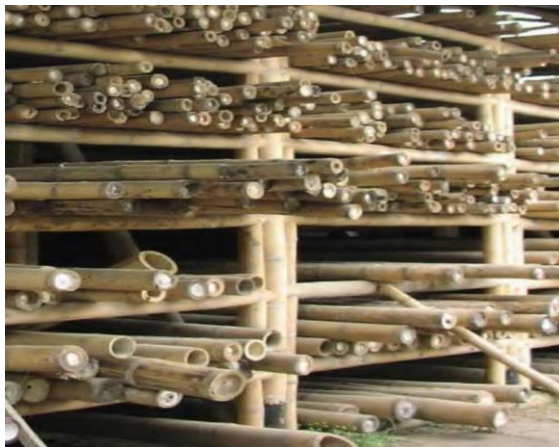
Plate 18: Bamboo drying shed
