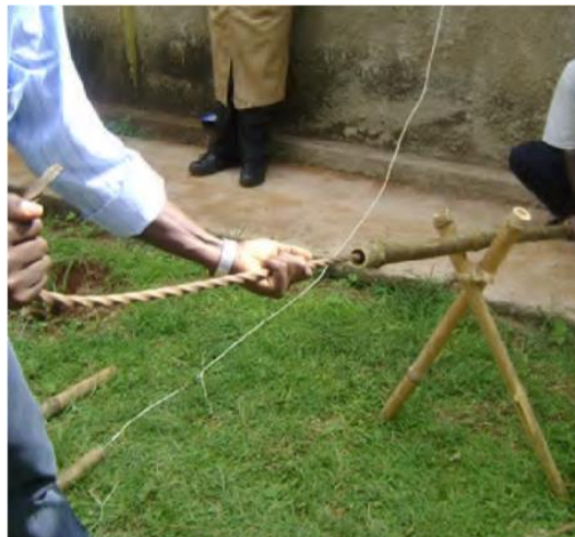
Plate 19: Perforating bamboo culms
