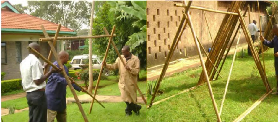
Plate 22: Drying bamboo culms away from direct sunlight
